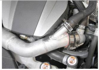
10. Install the intake pipe onto the coupler previously installed. Connect the breather hose to the port on the new intake pipe.
