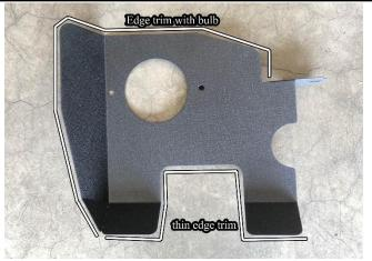
12. Install 25" of the provided edge trim on the top and 18" onto the bottom of the heat shield.
