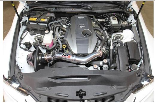
16. Re-connect the MAF sensor wiring. Reinstall the factory trim pieces to complete the installation. NOTE: If installing onto an Lexus RC200T or RC300, the passenger side trim piece will need to remain off.
