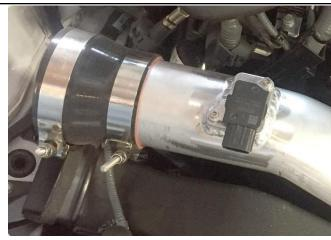
11. Install the hump coupler onto the end of the intake pipe. Transfer the MAF sensor over from the factory air box and secure it using the Allen screws provided.
