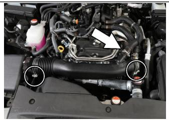
4. Loosen the hose clamps securing the intake tube from the air box and the turbo inlet.
