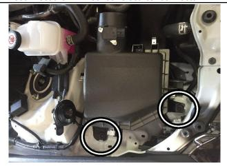
8. Remove the two bolts indicated in the image. You may remove the factory air box from the engine bay.
