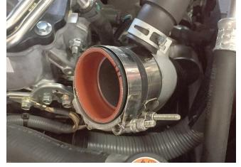
9. Install the silicone coupler along with the two smaller T-bolt clamps onto the stock turbo inlet pipe.
