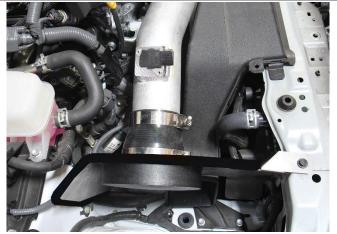
14. Install the heat shield onto the vehicle by inserting the small side of the venturi into the reducer coupler on the intake pipe.
