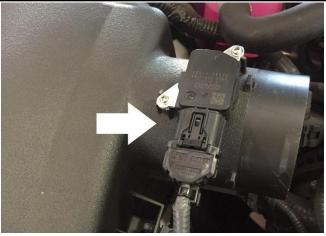
6. Disconnect the MAF sensor electrical connector.
