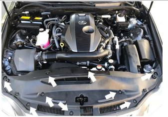
3, Remove the 9 push clips on the panel located at the front of the vehicle by pushing in at the center of the clips. Once removed, you may put the panel aside for use later.
