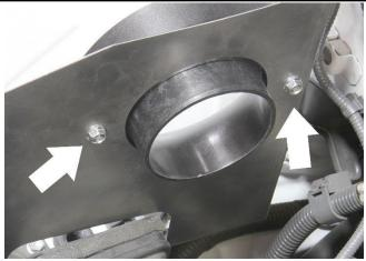
13. Install the venturi onto the heat shield and secure it using two M6 bolts and washers provided in the hardware packet.
