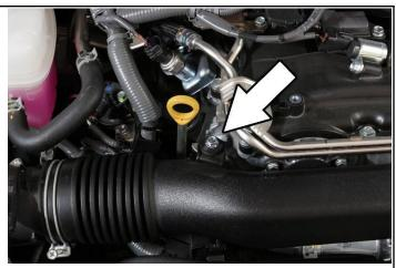
5. Remove the 10mm bolt securing the intake tube bracket. Remove the stock intake tube from the engine bay.
