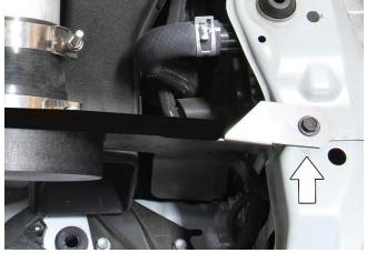
15. Remove and reinstall the bolt on the radiator support to secure the heat shield to the vehicle.
