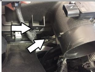
7. Unclip the electrical wiring from the factory air box.
