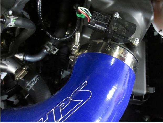
4. Install the HPS silicone intake hose along with the T-bolt clamps.
