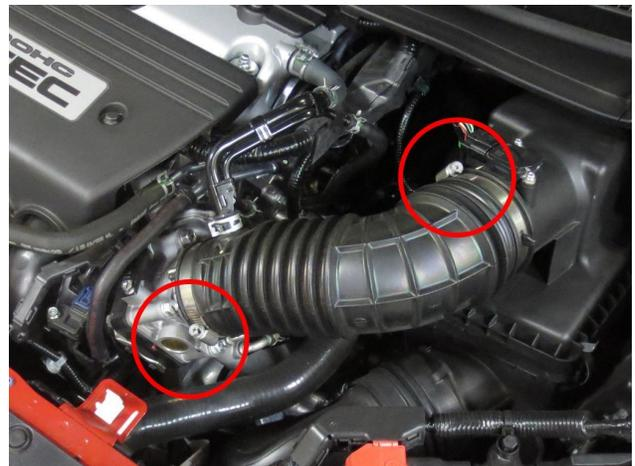
3. Loosen the two hose clamps and remove the intake hose. When pulling out the hose, push the coolant hose out of the retaining clip.
