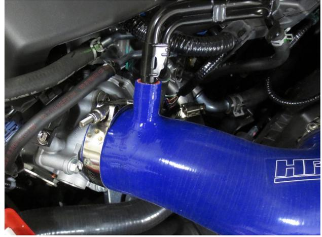
5. Reconnect the breather hose. Connect and tighten the clamps at the throttle body and filter side.
