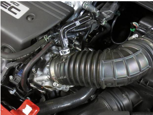
2. Disconnect the breather hose from the stock intake tube.
